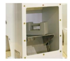
The calibration is performed on site by placing a standard weight on the flow sensor. The system is precalibrated in the factory thus requiring just a few easy actions for reajusting. Through an external adjusting screw it is possible to modify the inclination of the tray in order to obtain the pre-set weight value.
