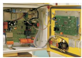
Developed with the latest technology in electronics components, it is fully integrated and easily accessible for maintenance and wiring. The detecting of the impact force is done through top performance A/D converter used in the weighing systems. Input and output are protected from any wiring error and from electromagnetic noises, making these instruments really industrial.
