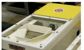
The pneumatic drive guarantees high operator security and, in case of electric black-out, a quick putting in closing position. Wiring, electric panel and electronic components have been designed to pass any standard tests. On request a version of DPM according to ATEX standards for use in area 22, certified by German TÜV, is available.
