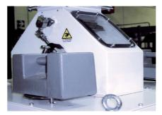
Calibration and periodical check can be easily and quickly executed by placing standard weights on the disks assembled to the weighing hoppers. Commands given through the operator panel allow to perfectly readjust the machine obtaining the required accuracy for effective control of plant yield.
