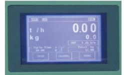
The use of touch-screen display make the operator interface extremely logical and user-friendly. Few and simple pressures on virtual buttons permit setting of main working parameters and detecting possible alarms. The head page reports evidently the decisive flow rate, net hopper weight and basic using indications.
