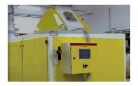
The double hopper arrangement allows higher production and weighing with a lower volume than any other solution. This scale is particularly appreciated in plants requesting high performance in limited space. The weight measurement is obtained in a closed environment so giving results of maximum precision as it is not affected by external disturbance or pressure balance above and beneath weighing hoppers.
